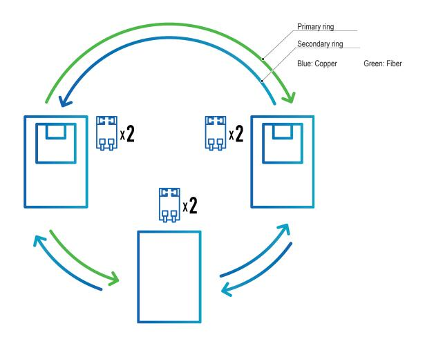
EBL512 G3 can be used as a stand-alone CIE or connected in a redundant network of up to 30 control units in a wide distribution throughout the premises The network is of multi master type, which means that all information is available to all CIE and the whole system can be controlled from any of the control units in the network
