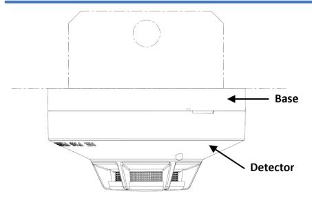
Each 4W-882 detector is used with a mounting base (B801R) that permits the detector to be mounted directly to a 50 or 60mm junction box as the left figure showed.
